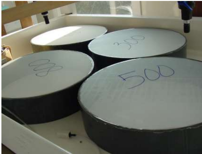
Figure 6: Mesh sieves that act as downweller setting bins.
