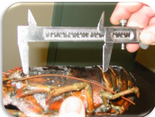
Photo: Caliper being used to measure the carapace of a lobster.
